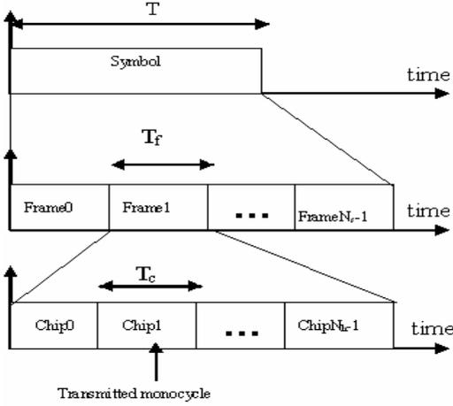
Fig.1. Frame structure for time hopping signals
