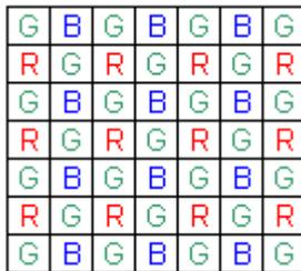
Figure 1: Typical Bayer pattern used in single-CCD digital cameras.
