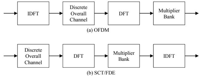
Fig. 1. Transmit and receive block diagrams of OFDM and SCT/FDE.
