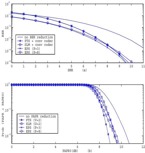
Figure 2: BER and CCDF of PAPR for EPS, PTS and SLM
