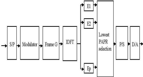
Figure 1: Transmitter for EPS scheme
