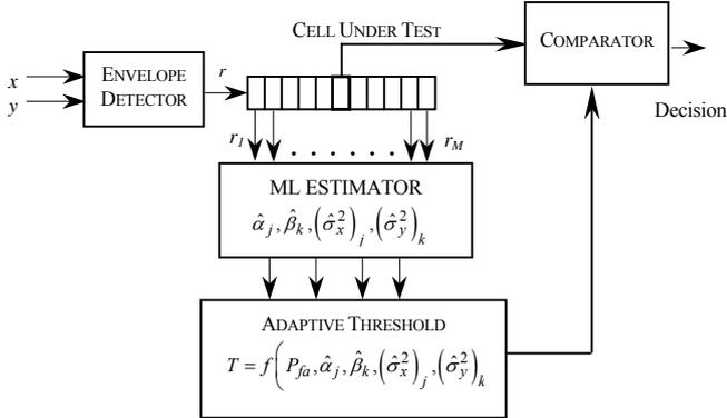
Figure 1. ML-CFAR structure.
