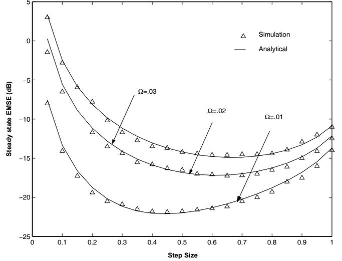
**Fig. 1.** Analytical and experimental  $\zeta$  for  $\Omega = 0.01$ ,  $\Omega = 0.02$  and  $\Omega = 0.03$ , and  $tr\{\mathbf{Q}_n\} = 10^{-7}$ .
