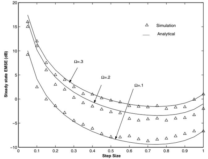
**Fig. 3.** Analytical and experimental  $\zeta$  for  $\Omega = 0.1$ ,  $\Omega = 0.2$  and  $\Omega = 0.3$ , and  $\text{tr}\{\mathbf{Q}_n\} = 10^{-2}$ .
