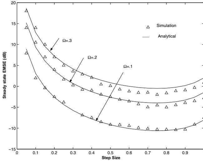
**Fig. 2.** Analytical and experimental  $\zeta$  for  $\Omega = 0.1$ ,  $\Omega = 0.2$  and  $\Omega = 0.3$ , and  $\text{tr}\{\mathbf{Q}_n\} = 10^{-7}$ .
