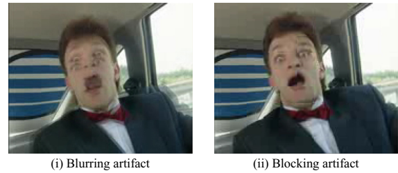
Figure 2: Visual artifacts in motion compensated frame rate up conversion
