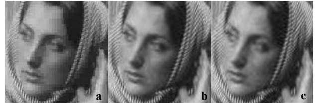
Figure 4: Coding performances for Barbara image and Daubechies wavelet filters; a : db1, b :db7, c :db40
