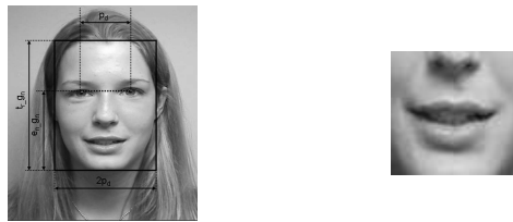
Figure 2: Anthropometric measures used for locating the lower face region from the pupils' distance (a), and the cropped ROI (b).
