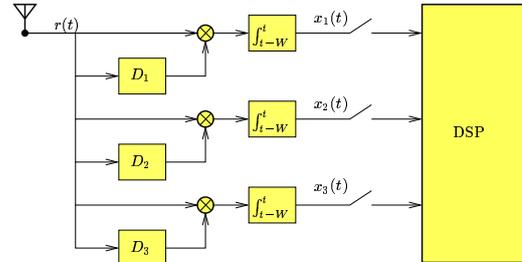
Figure 1: The structure of the autocorrelation receiver.
