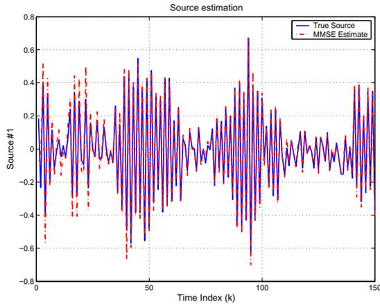
Figure 3: Source estimation for SIMO system
