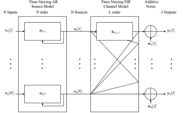
Figure 1: Graphical representation of state space model
