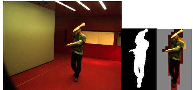
Fig. 7: Shape-oriented preprocessing for H.264/AVC.
