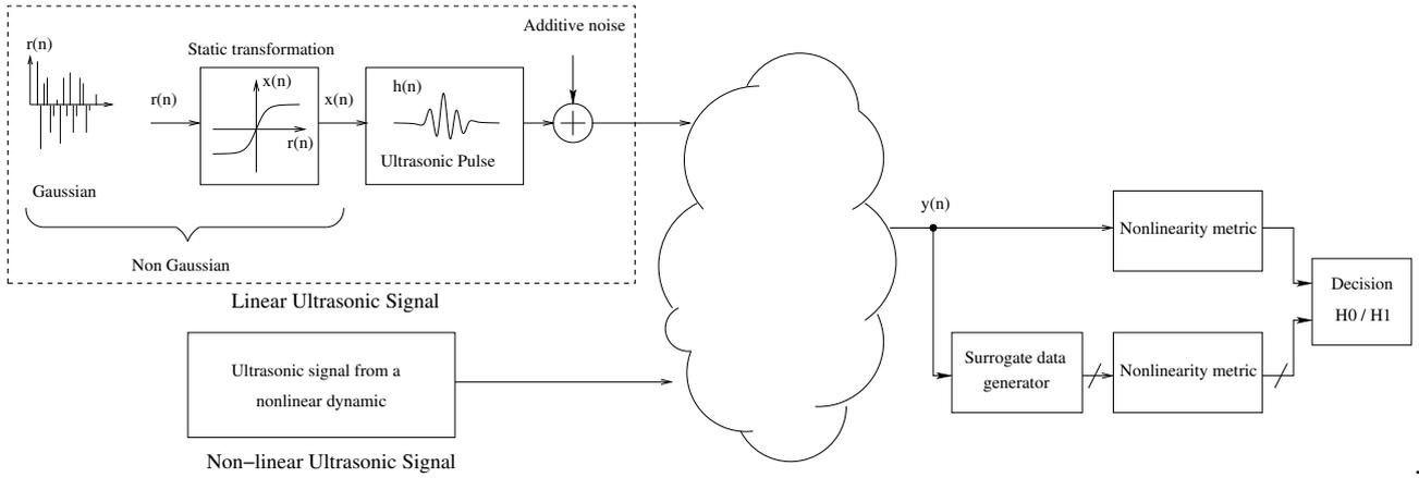
Figure 2: Proposed algorithm for bubble detection on ultrasonic signals
