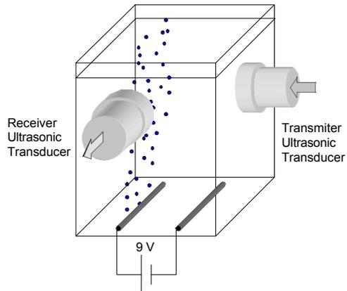
Figure 3: Electrolysis generation of bubbles and transducer layout
