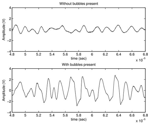
Figure 4: Signals acquired with and without bubble presence
