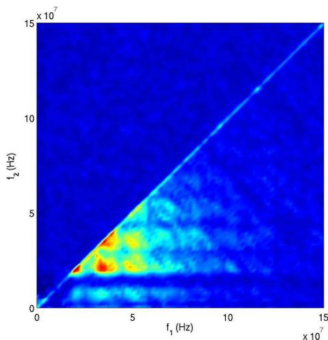
Figure 6: Bicoherence estimation of the signals when bubbles are not present (upper diagonal) and when bubbles are present (lower diagonal)
