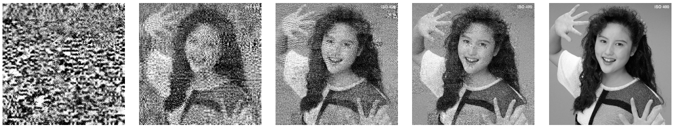
(a) Reconstructed image. m = 1 . (PSNR 6.8dB) (b) Reconstructed image. m = 2 . (PSNR 10.4dB) (c) Reconstructed image. m = 3 . (PSNR 12.3dB) (c) Reconstructed image. m = 4 . (PSNR 15.6dB) (d) Reconstructed image. m = 5 .(Lossless)
