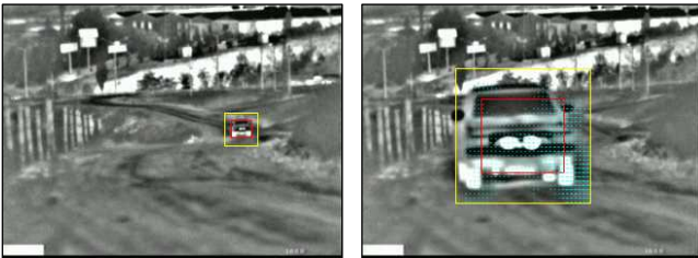
Figure 8. The 1 st (left) and 736 th (right) frames of the Pursaklar-1b Sequence. Demonstration of target size adaptation of the CDWT-based tracking algorithm.
