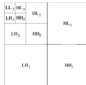
Figure 1: Three levels discrete wavelet decompositions.
