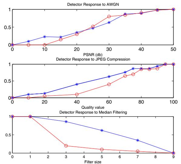
Figure 2: The comparison of the proposed method and the method in [4] under AWGN, JPEG compression and median filtering. The plots with '\*' corresponds to the proposed algorithm.
