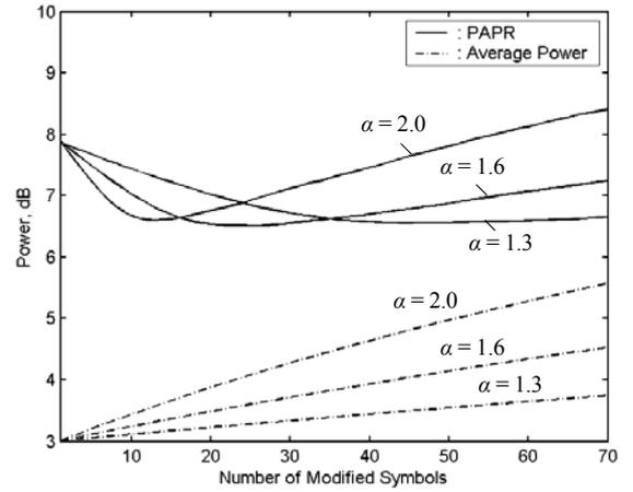
Fig. 2. PAPR and average power vs. number of modified symbols for different scaling factors.
