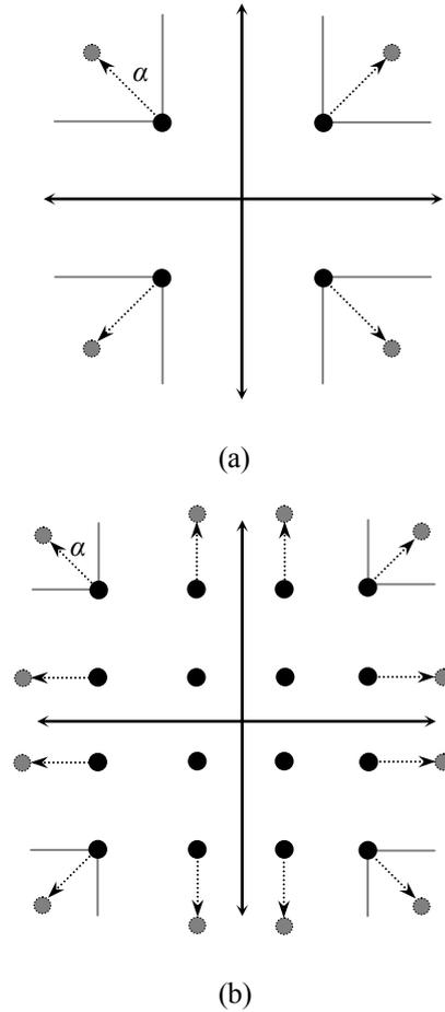
Fig. 1. Dynamic constellation shaping with scaling factor  $\alpha$ : a) QPSK, b) 16-QAM.
