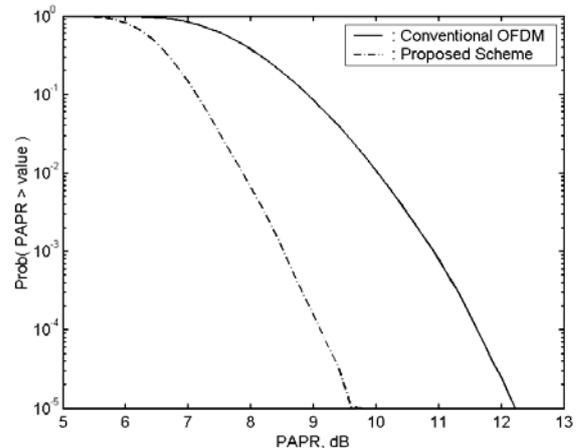
Fig. 3. CCDF of PAPR for conventional OFDM and the proposed scheme.
