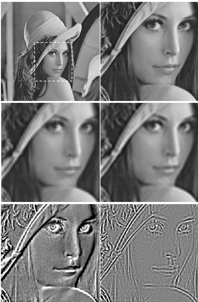
Figure 4. Extract from original Lena image (top), 4x reconstructions using bilinear interpolation (mid. left) and the proposed method (mid. right) and corresponding amplified error images (bottom).
