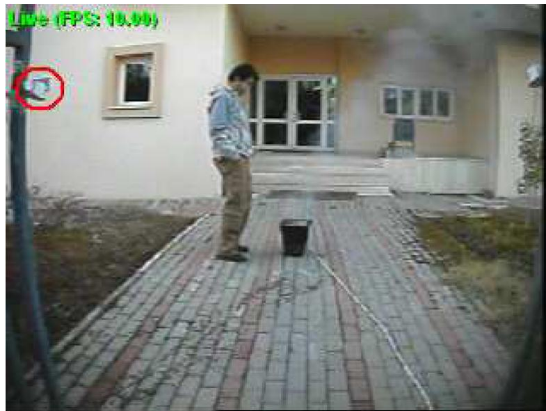
Figure 4.12: The PIR sensor is encircled. The fire is close to die out completely. A man is also within the viewing range of the sensor. No false alarm is issued for this case.
